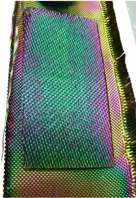
Figure 3: BN Coating on CG-Nicalon Fabric on T300 Fabric (underneath).
